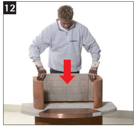
12 Mount back part of the 3-piece fireproof insert of the firebox. Take care that you have a distance to the firebox of approx. 1/4"
